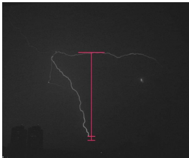
Fig. 5 Estimation of horizontal channel propagation height H .
